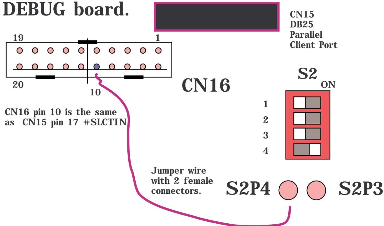
Turn ON S2 pin 4 to ground CN 16 pin 10 & CN15 pin 17
